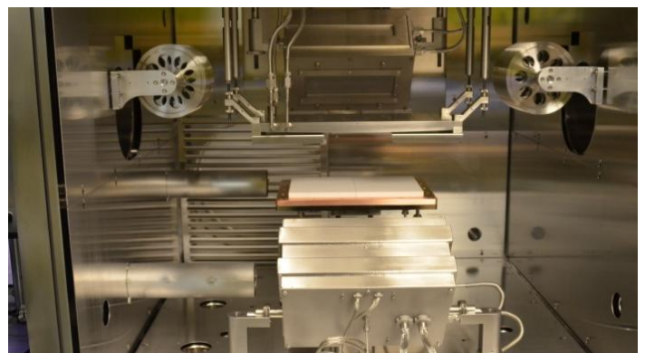
Inside view of IBAD System with two 6 x 22 cm RF ion Sources and Multi-Pass Configuration.
